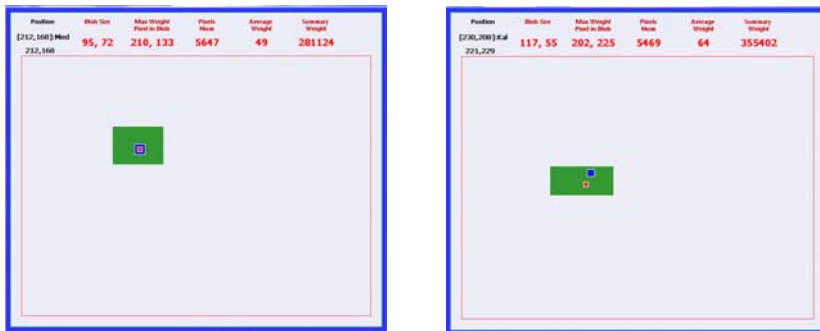
Fig.3. Result of Applying (Left)Median and (Right) Kalman Filters for Blob Center illustration
